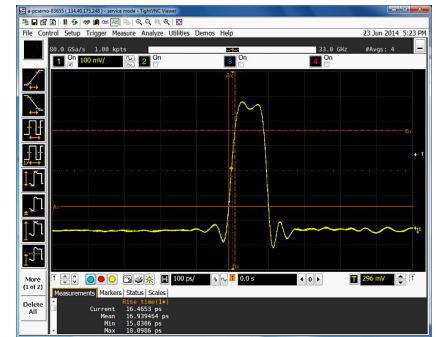
Figure 5. 100 ps pulse with 17 ps risetime.
